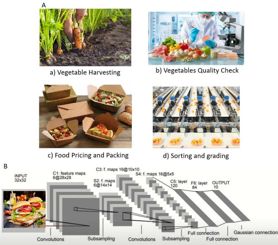
Figure 7 Computer vision and AI driven food industry (A) harvesting, picking, quality control and sorting using vision algorithms, and (B) LeNet deep learning architecture for food classification
